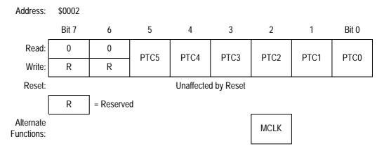
Figure 23-8. Port C Data Register (PTC)
