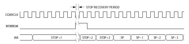
Figure 7-16. Stop Mode Recovery from Interrupt or Break
