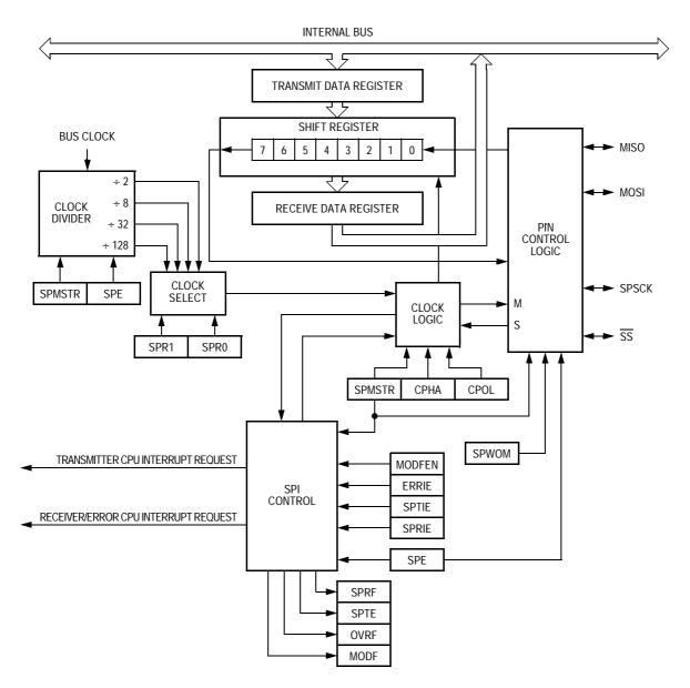
Figure 17-1. SPI Module Block Diagram
