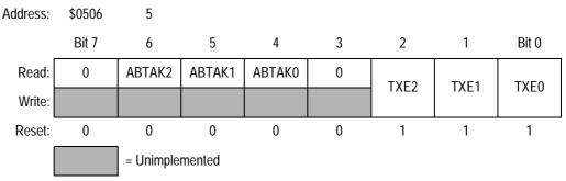
Figure 24-21. Transmitter Flag Register (CTFLG)
