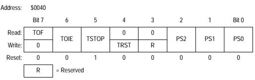
Figure 19-4. TIMB Status and Control Register (TBSC)
