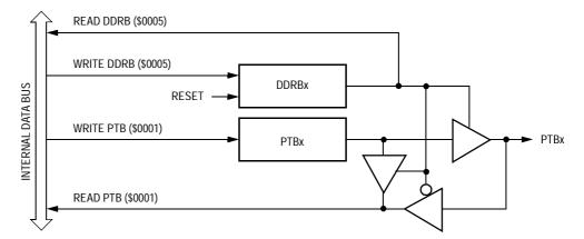
Figure 23-7. Port B I/O Circuit
