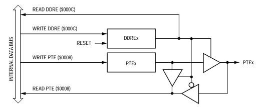
Figure 23-16. Port E I/O Circuit
