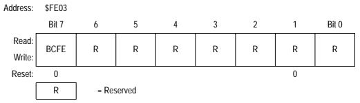
Figure 7-19. SIM Break Flag Control Register (SBFCR)
