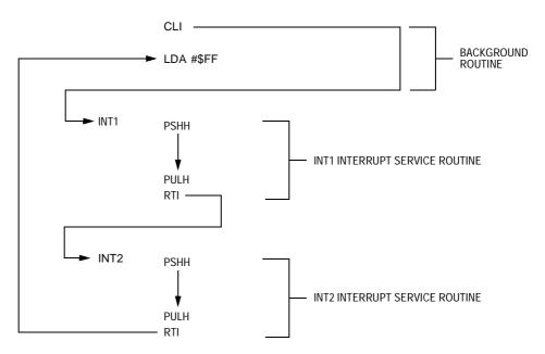
Figure 7-11. Interrupt Recognition Example
