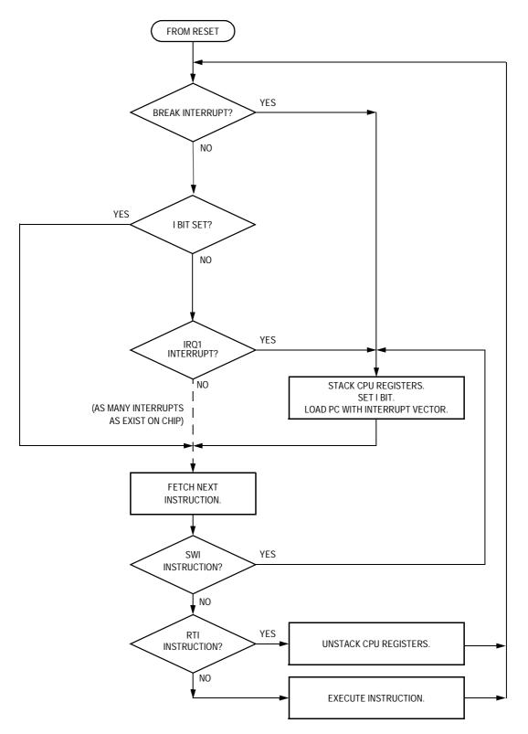
Figure 7-9. Interrupt Processing
