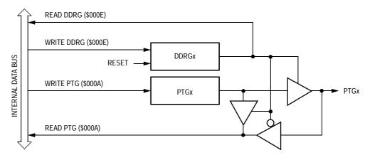
Figure 23-22. Port G I/O Circuit
