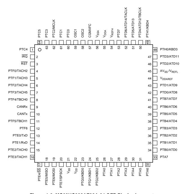
Figure 1-2. MC68HC908AZ32A 64 QFP Pin Assignments
