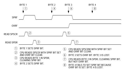
Figure 17-6. Missed Read of Overflow Condition
