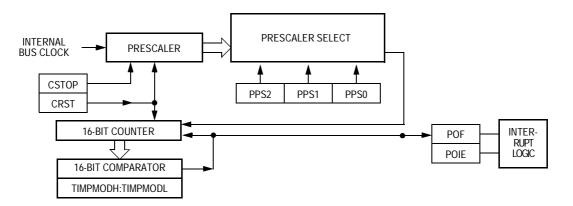
Figure 20-1. PIT Block Diagram
