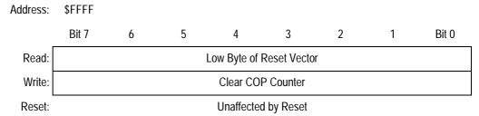
Figure 13-2. COP Control Register (COPCTL)
