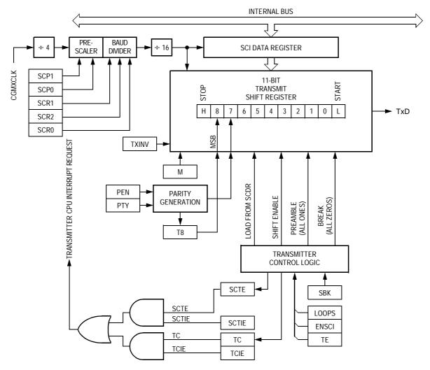
Figure 16-4. SCI Transmitter
