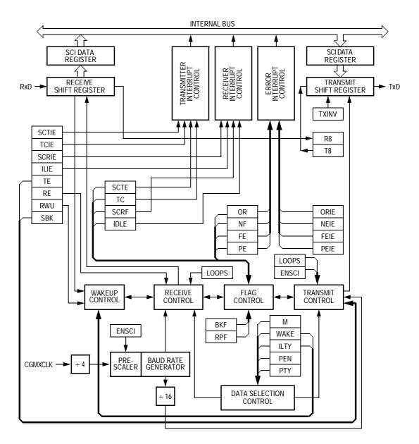
Figure 16-1. SCI Module Block Diagram
