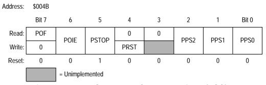
Figure 20-3. PIT Status and Control Register (PSC)
