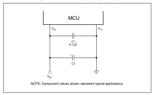
V<sub>SS</sub> is also the ground for the port output buffers and the ground return for the serial clock in the Serial Peripheral Interface module (SPI). See Section 17. Serial Peripheral Interface (SPI).
