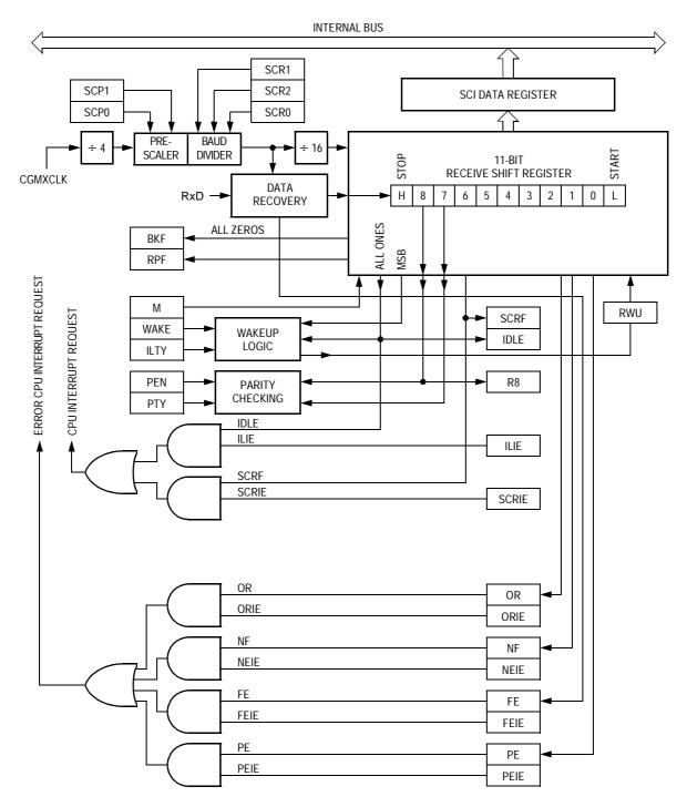
Figure 16-6. SCI Receiver Block Diagram
