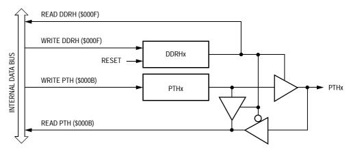
Figure 23-25. Port H I/O Circuit
