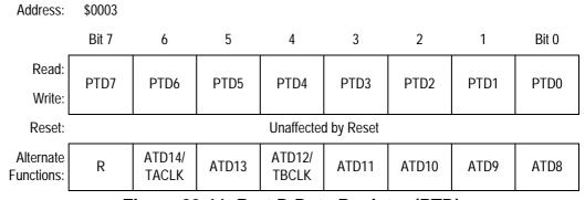
Figure 23-11. Port D Data Register (PTD)
