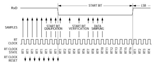
Figure 16-8. Receiver Data Sampling
