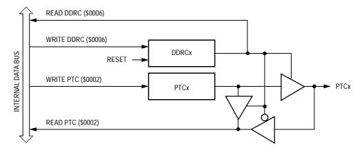
Figure 23-10. Port C I/O Circuit
