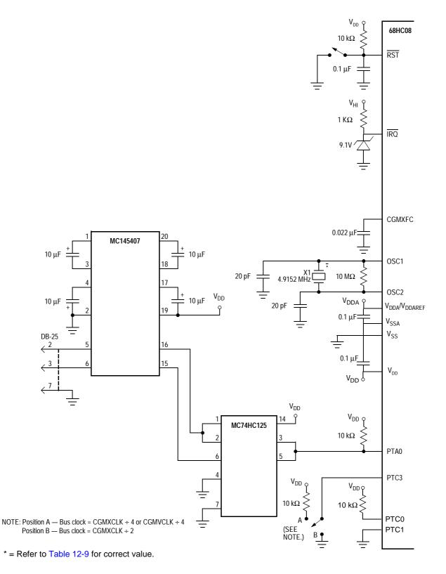
Figure 12-1. Monitor Mode Circuit
