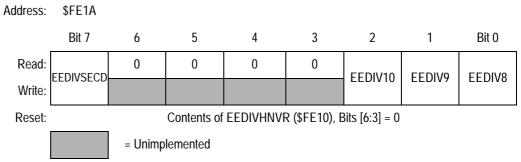
Figure 5-5. EEDIV Divider High Register (EEDIVH)
