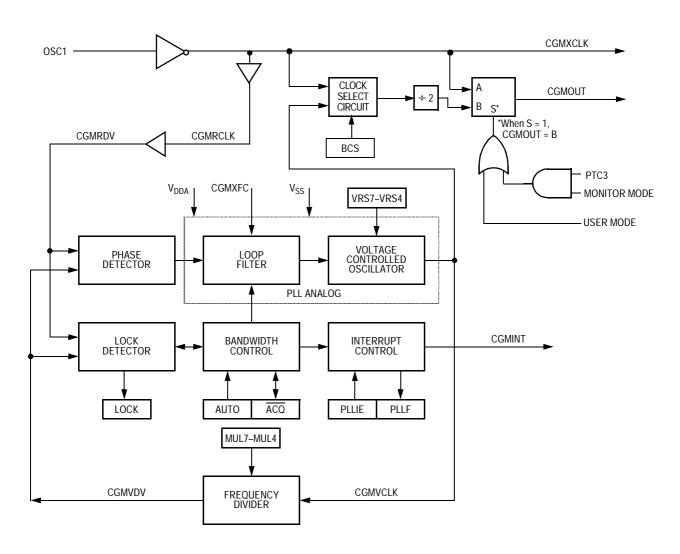
Figure 8-1. CGM Block Diagram
