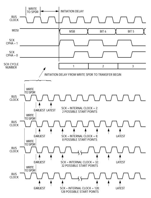
Figure 17-5. Transmission Start Delay (Master)
