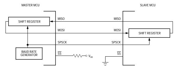
Figure 17-2. Full-Duplex Master-Slave Connections
