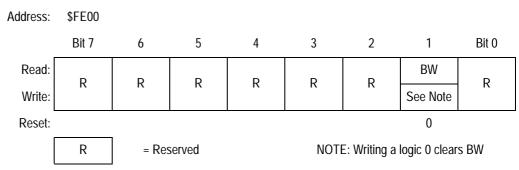
Figure 7-17. SIM Break Status Register (SBSR)
