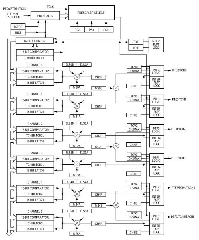
Figure 18-1. TIMA Block Diagram
