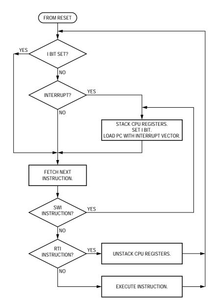
Figure 15-2. IRQ Interrupt Flowchart
