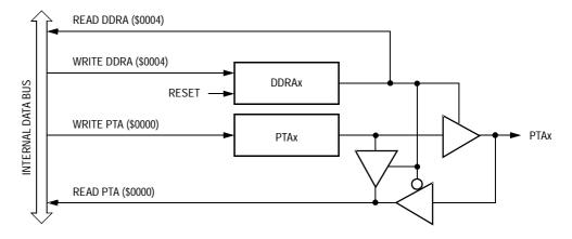
Figure 23-4. Port A I/O Circuit
