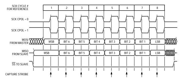
Figure 17-3. Transmission Format (CPHA = 0)
