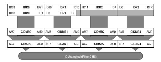
Figure 24-3. Single 32-Bit Maskable Identifier Acceptance Filter
