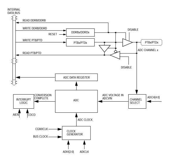
Figure 21-1. ADC Block Diagram
