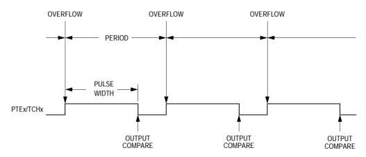
Figure 18-3. PWM Period and Pulse Width
