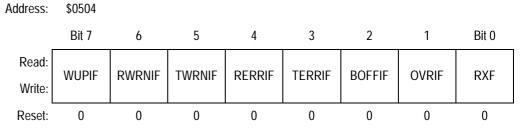
Figure 24-19. Receiver Flag Register (CRFLG)
