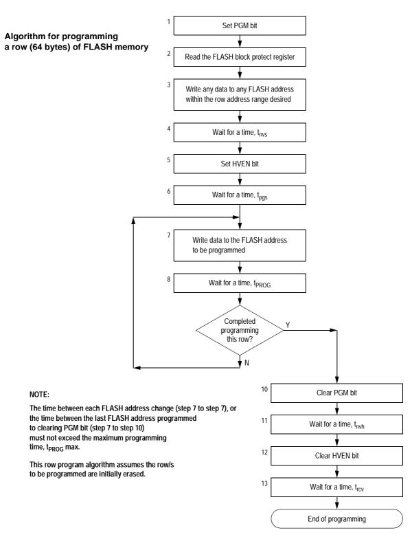
Figure 4-4. FLASH Programming Algorithm Flowchart
