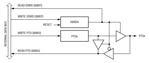
Figure 23-13. Port D I/O Circuit
