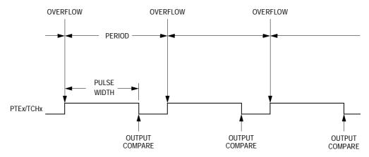
Figure 19-3. PWM Period and Pulse Width
