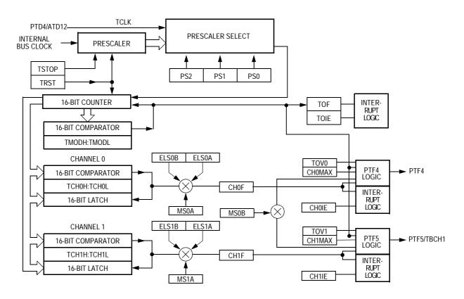
Figure 19-1. TIMB Block Diagram
