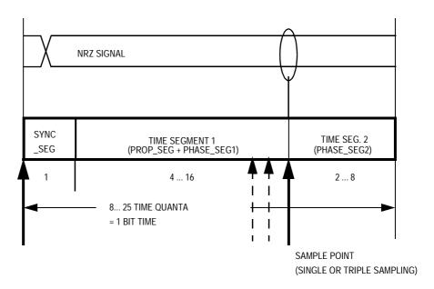
Figure 24-8. Segments within the Bit Time
