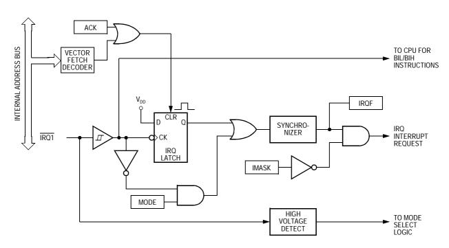
Figure 15-1. IRQ Block Diagram
