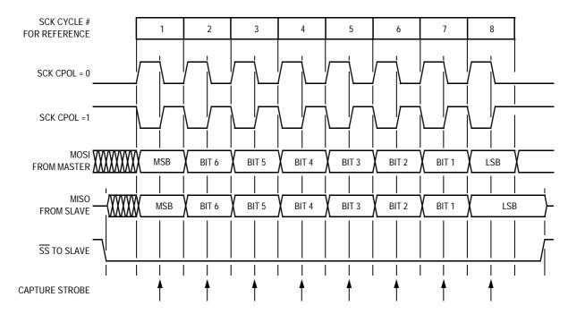
Figure 17-4. Transmission Format (CPHA = 1)
