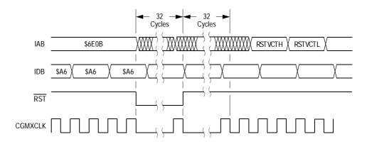
Figure 7-14. Wait Recovery from Internal Reset
