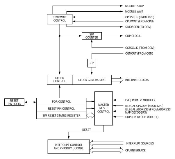
Figure 7-1. SIM Block Diagram
