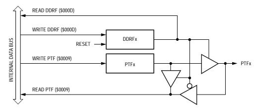
Figure 23-19. Port F I/O Circuit
