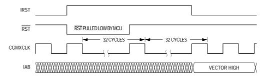
Figure 7-5. Internal Reset Timing
