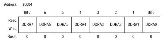
Figure 23-3. Data Direction Register A (DDRA)
