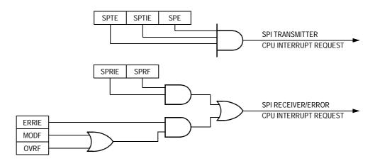
Figure 17-8. SPI Interrupt Request Generation
