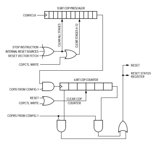
Figure 13-1. COP Block Diagram
