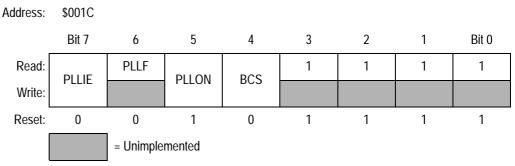
Figure 8-4. PLL Control Register (PCTL)
