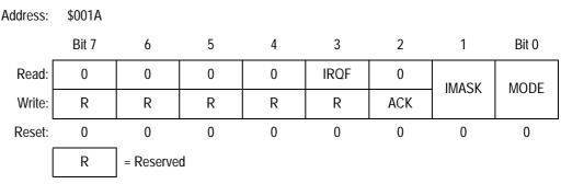
Figure 15-3. IRQ Status and Control Register (ISCR)
