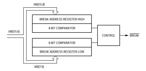
Figure 11-1. Break Module Block Diagram
